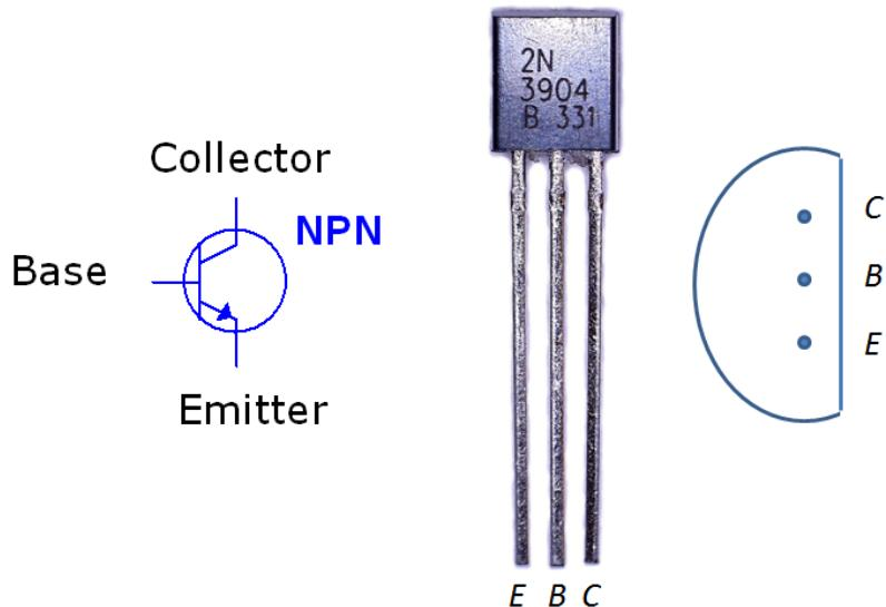
2. Is it possible to distinguish the emitter from the collector using only a multimeter? Yes, but only barely. (I will accept if you said no.) The base-collector junction has a slightly lower resistance.
